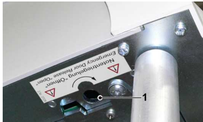
Fig. 7.2: Opening for the emergency lid release at the bottom of the centrifuge
