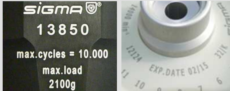
Fig. 3.1: Different service life – engraving on the bucket/rotor
